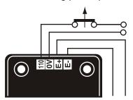
The exciter is switched off by disconnecting the AVR power supply (1 wire - 0 or 110V).
